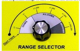
*RANGE: Ohms, KOhms, MOhms*Which area is the switch in? This information will help the operator in completing the formula for Ohm-cm. Each position of the switch shows the *RANGE*, as well as the multiplier for that *RANGE*.
