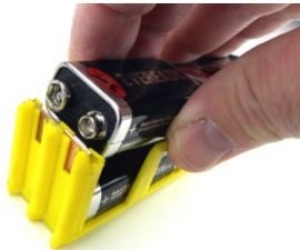
Figure 6 – slide battery in observing polarity
