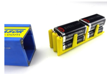
Figure 16 – slide battery sled back into case, closed end first
