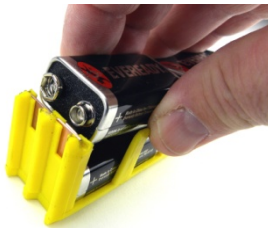
Figure 14 – slide battery in observing polarity
